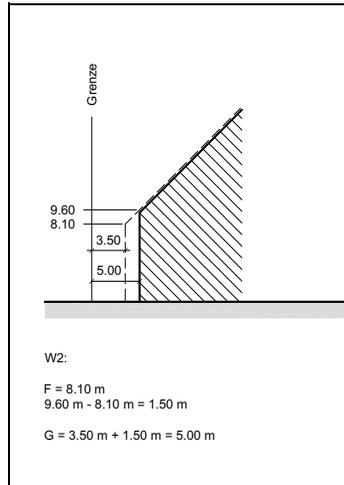
**Figur 7.12 Fassadenlänge (§ 260 PBG / § 27 ABV)**
