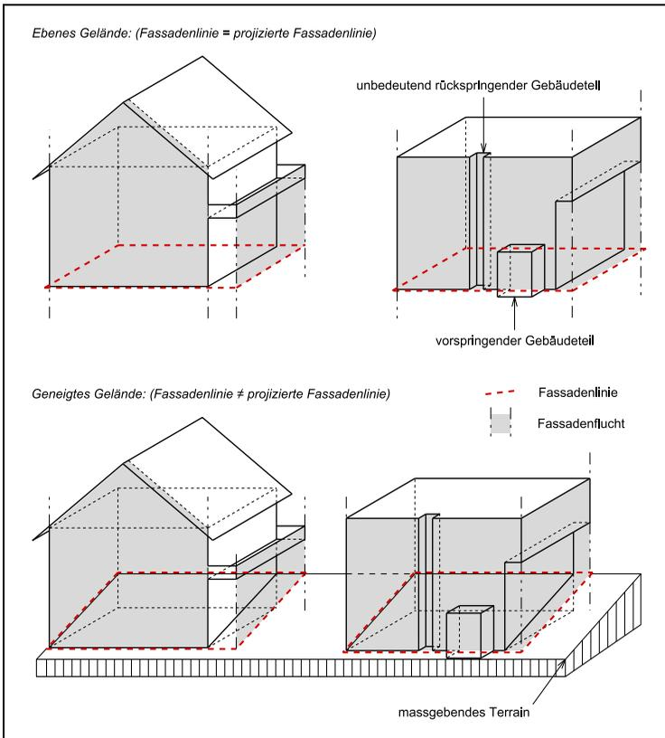
**Figur 3.3 Projizierte Fassadenlinie (§ 6 b ABV)**
