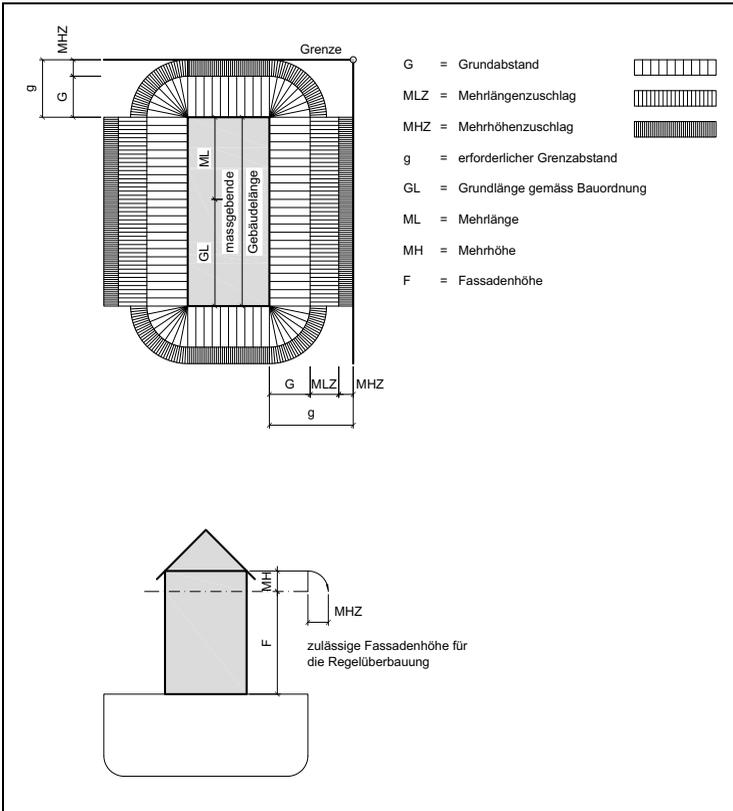
**Figur 7.6 Grenzabstand bei gestaffelten Fassaden (§§ 21–26 ABV)**
